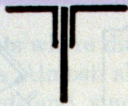
(a) Top Chord (b) Bottom Chord (c) Bottom Chord Sections for Members subjected to Bending Stress
