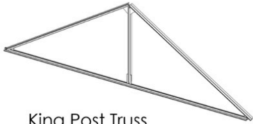
King Post Truss
