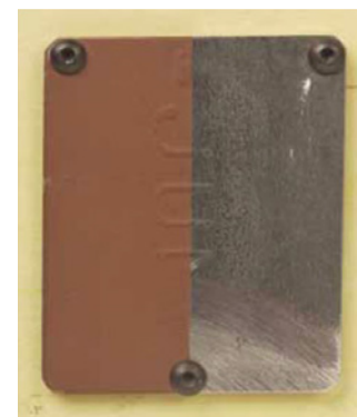
57 Fig. 3.1 Mill marks removed. (Courtesy of AISC)
