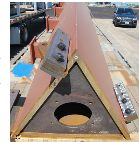
The Bow Encana, Calgary uses an AESS 4 finish on the front two faces of this very large triangular section in order to achieve a very straight edge along the length of the member. As the rear face of the member will be hidden from view, it is finished as structural steel to save on fabrication costs. These members are shipped singly to prevent damage.
