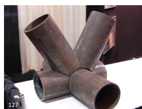
126 These tubular members were welded, using both tube-to-tube connections as well as X-shaped plate fabrications to resolve the geometry of the transition.
