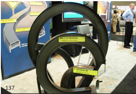
137 Although steel can be curved to very tight radii, it makes a difference if the steel shape is to be bent “the hard way” or “the easy way”. It will depend on the depth of the section and the curvature. If curves are very tight, some deformation is likely to occur. It is best to check with the fabricator early on in the design process when specifying curved steel.
