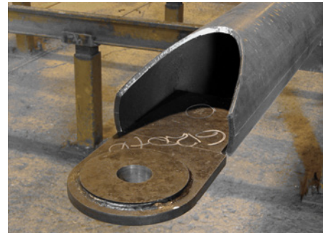
149 Several kinds of cuts are required to connect this plate to the HSS member to create a pin connection.
