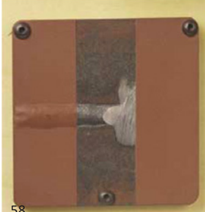
58 Fig. 3.2 Butt and plug welds ground smooth. Right side shows groove weld ground smooth. (Courtesy of AISC)
