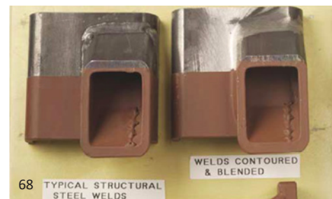
Fig. 4.2A Welds contoured and blended. The left-hand sample shows typical structural welds. The right-hand sample shows how they have been welded and contoured. (Courtesy of AISC)
