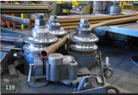
139 Steel bending is done at a special facility. The equipment and dies slowly push the steel into the desired curve after several passes through the machine.
