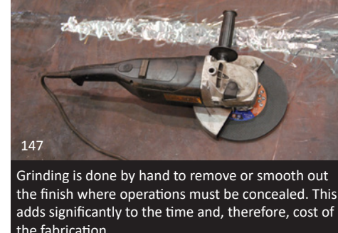
147 Grinding is done by hand to remove or smooth out the finish where operations must be concealed. This adds significantly to the time and, therefore, cost of the fabrication.
