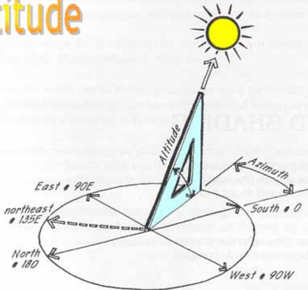
Figure 5.1: Solar azimuth and altitude angles. *Azimuth* angles are measured in each direction from south (for example, northeast = 135° E). *Altitude* angles are measured vertically from the horizon. (Reproduced from Moore, 1985, by permission.)
