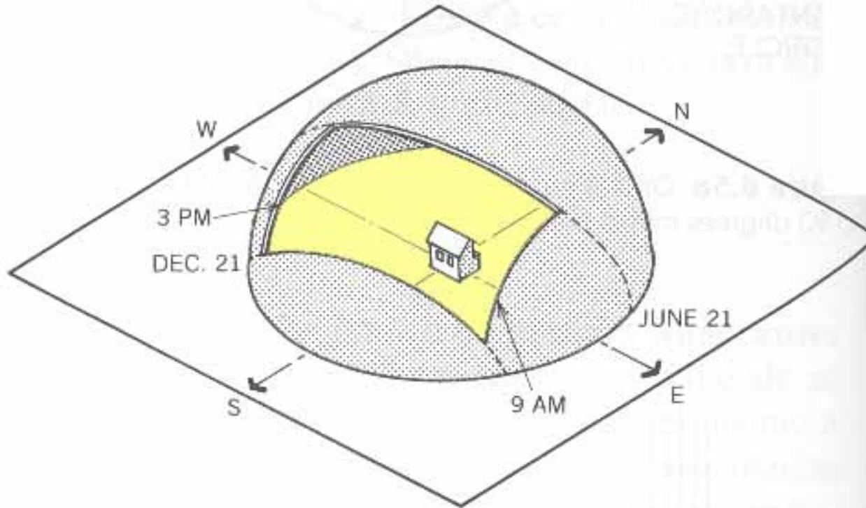
**Figure 6.8b** The solar window from about 9 A.M. to about 3 P.M.
