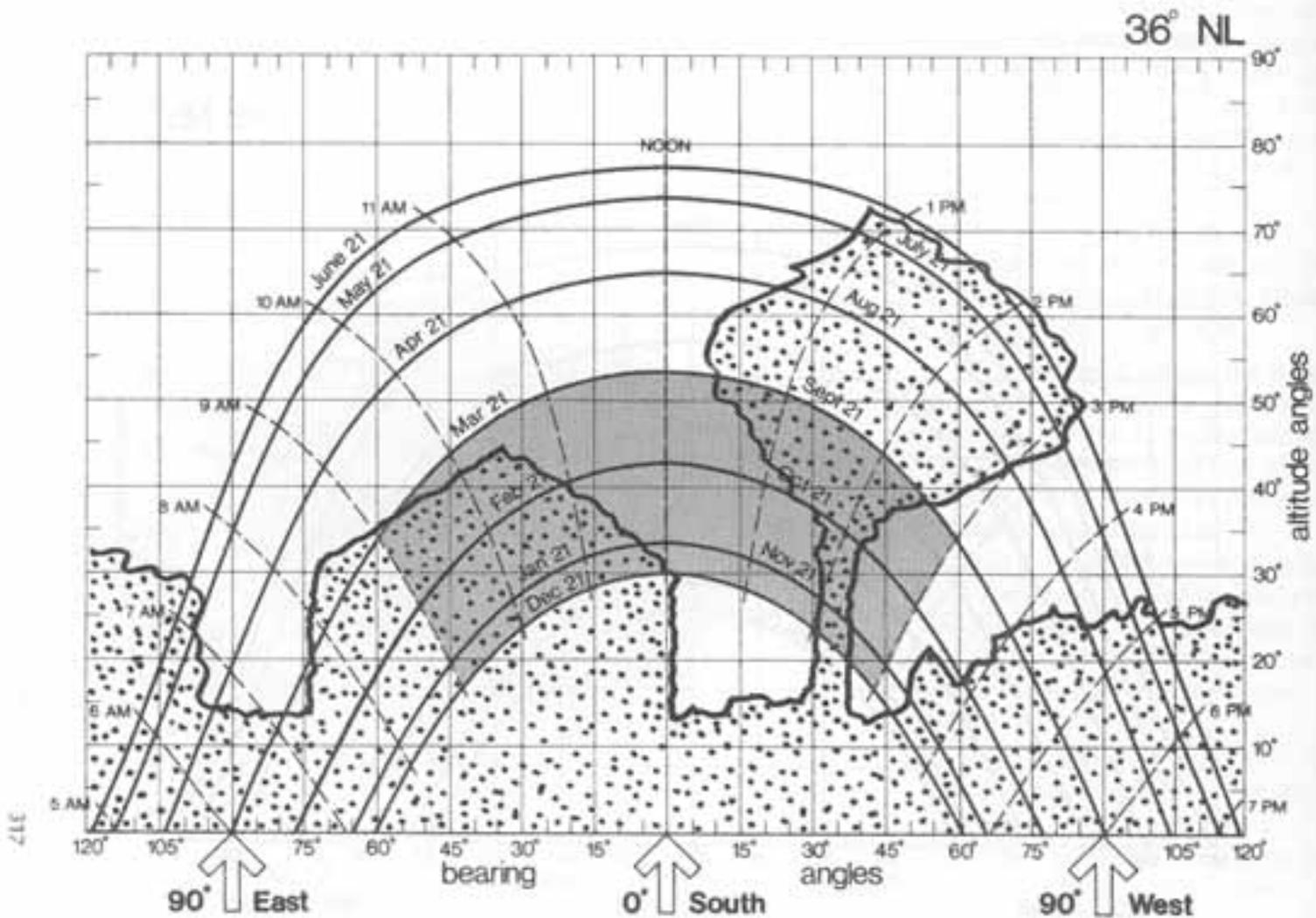
**Figure 6.12b** The winter solar window and silhouette of surrounding objects are shown on this vertical sun path diagram. The silhouette of a specific location was hand-drawn by means of a site-evaluator tool described in Section 6.14. (Sun path diagram from *The Passive Solar Energy Book*, copyright E. Mazria, 1979, reprinted by permission.)
