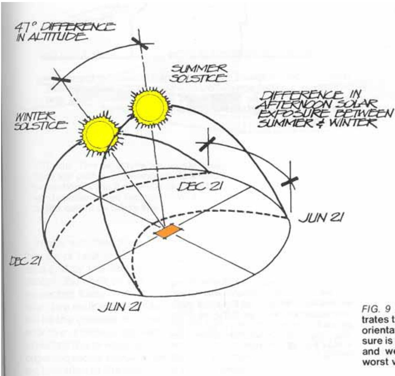
FIG. 9 Sunpath diagram illustrates that the only meaningful orientation for winter sun exposure is south. In summer, east and west exposures are the worst villains for overheating.
