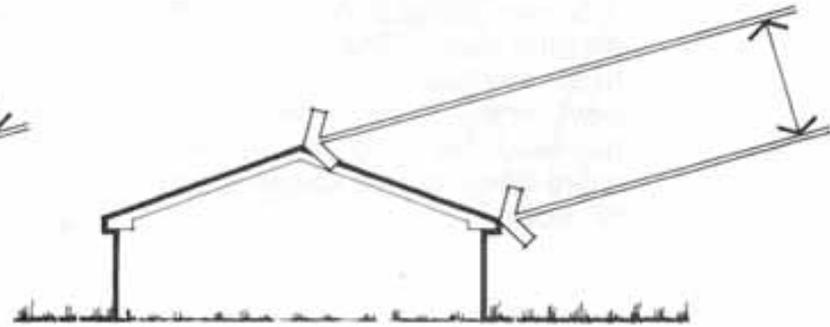
FIG. 12c. Roof shape has little effect on mid-day gain when sun is high.
