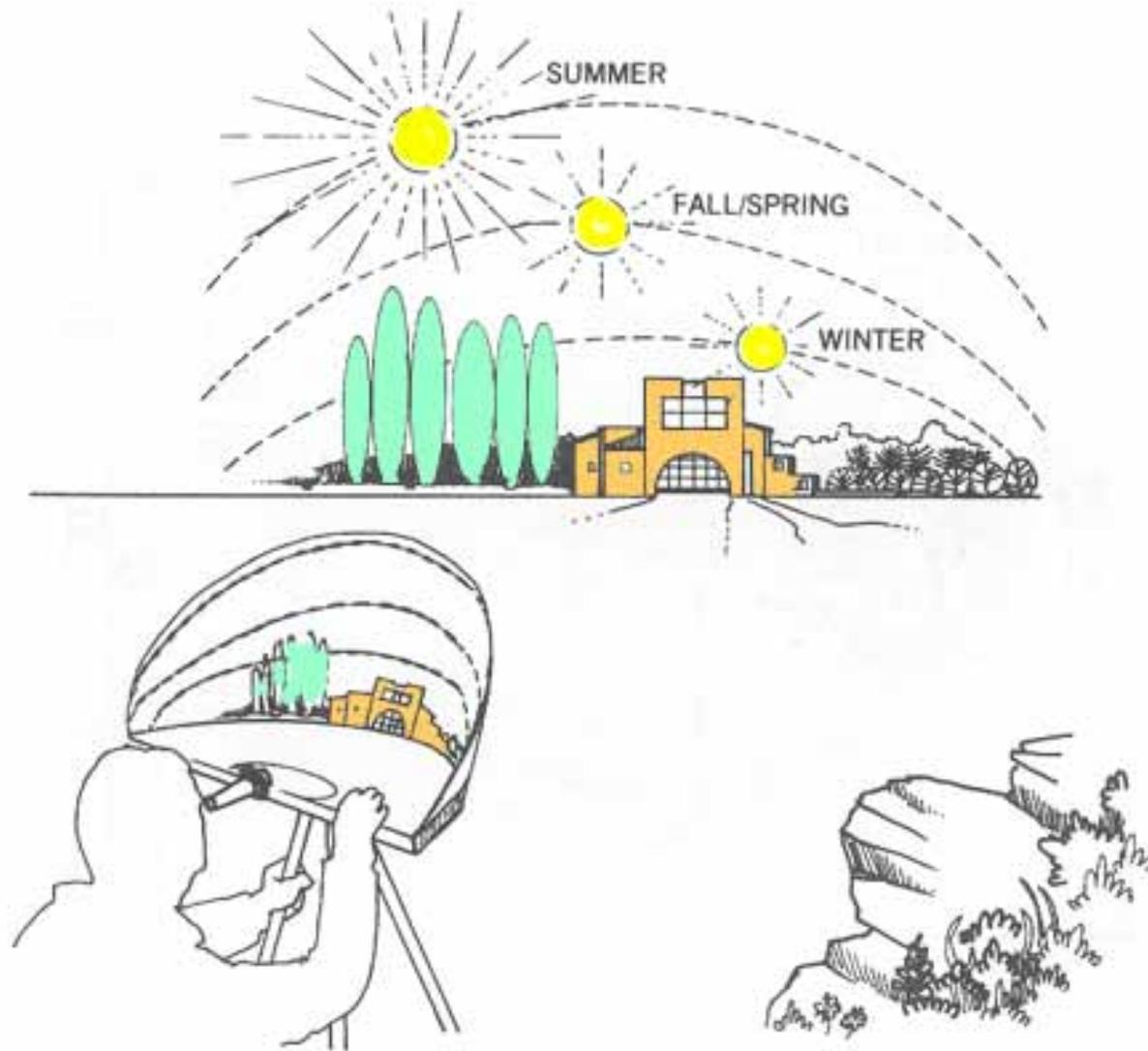
**Figure 6.14** The sun-path diagram used as part of a solar site-evaluation tool.
