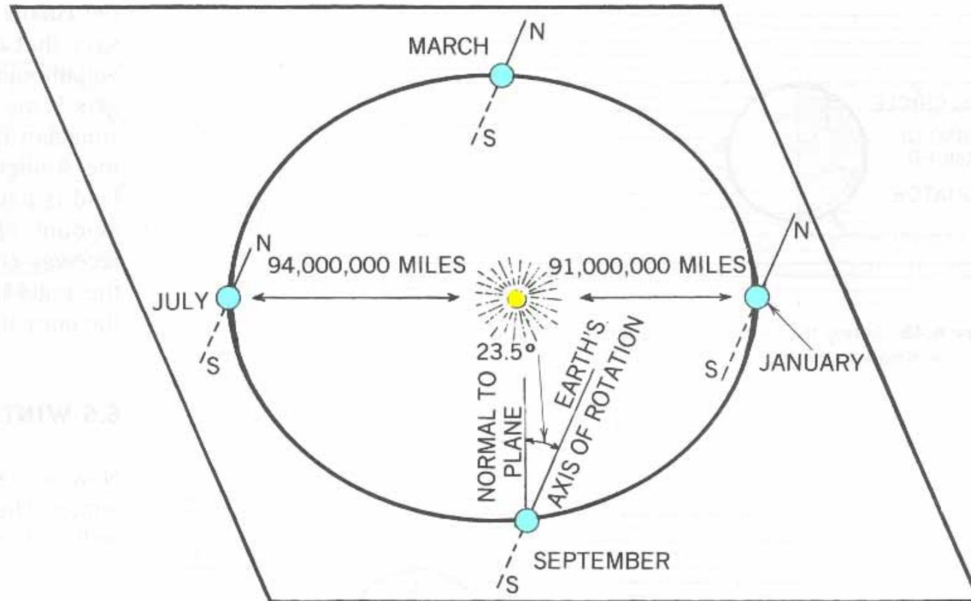
**Figure 6.3** The earth's axis of rotation is tilted to the plane of the elliptical orbit.
