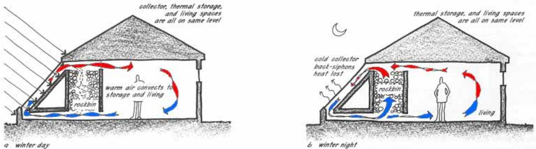
Figure 11.1: Positioning the collector, storage, and living areas at the same level in a convective air loop system: (a) winter day operation — level arrangement allows convective heating to occur during the day; (b) winter night operation — this "level" positioning of components permits unwanted back-siphoning, effectively cooling the system.
