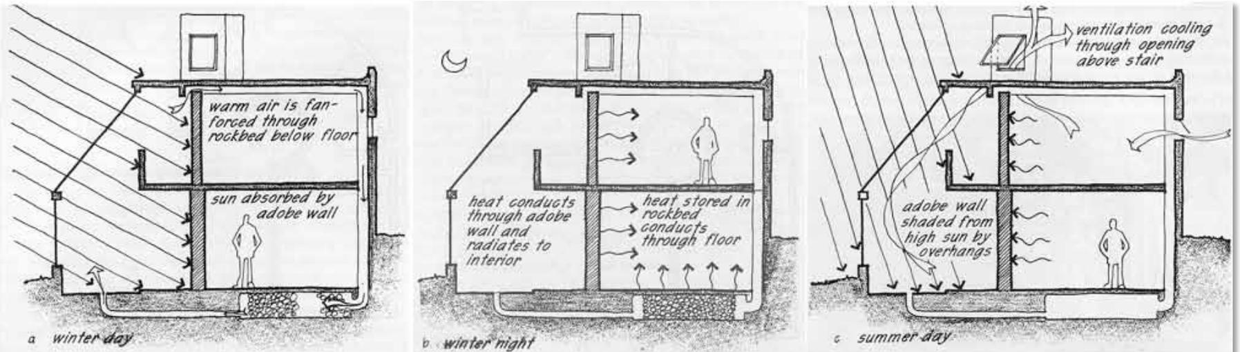
Figure 10.5: "Unit One" passive operation: (a) winter day, and (b) winter night. (Redrawn from Howard and Fraker, 1990, by permission.)
