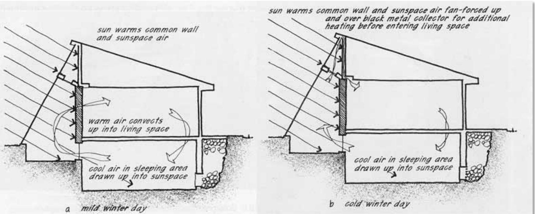
Figure 10.9: Solargreen passive operation: (a) winter day — passive heating only, and (b) winter day — with hybrid collector added.
