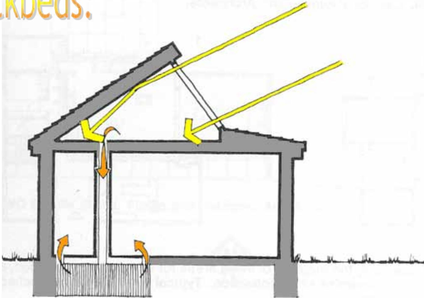
**FIG. 19e. Remote Gain and Storage**
