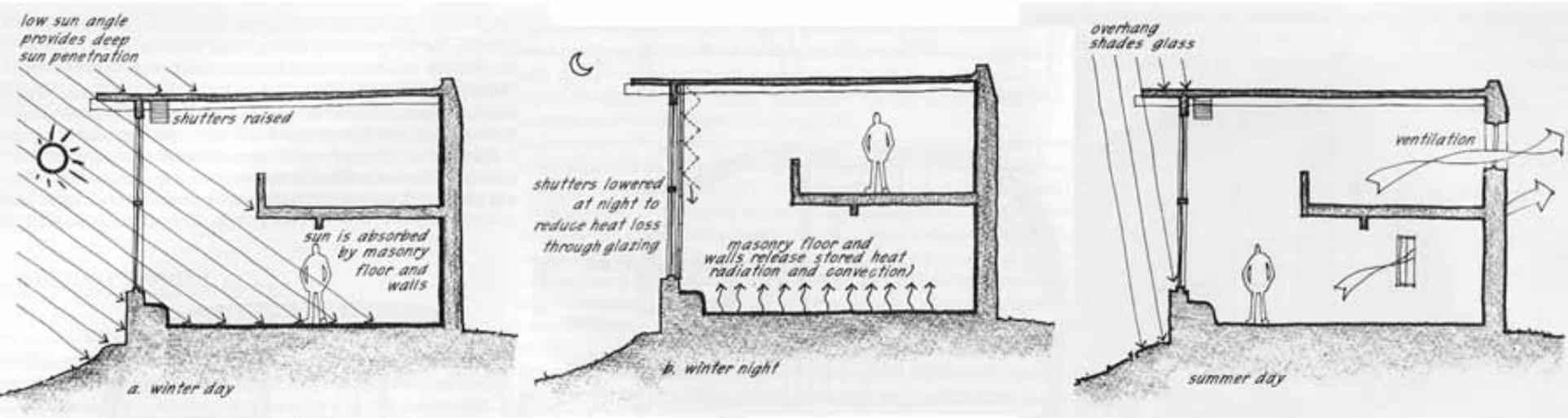
The direct gain system makes overt use of solar geometry to ensure that sun reaches the thermal mass in the winter, and that shading devices prevent solar access during the months where cooling is the dominant issue.
