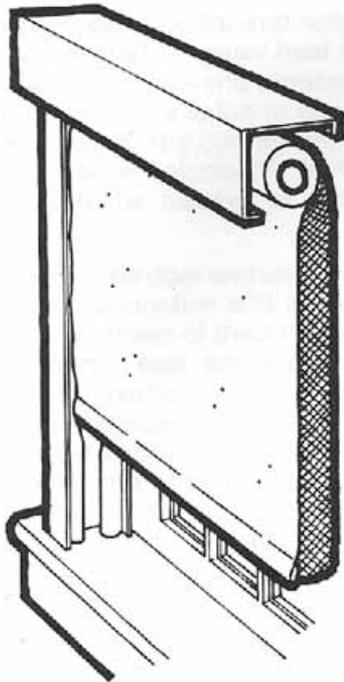
FIG. 39b. An insulating shade is designed to minimize conductive & radiative heat transmission, as well as a seal against infiltration.
