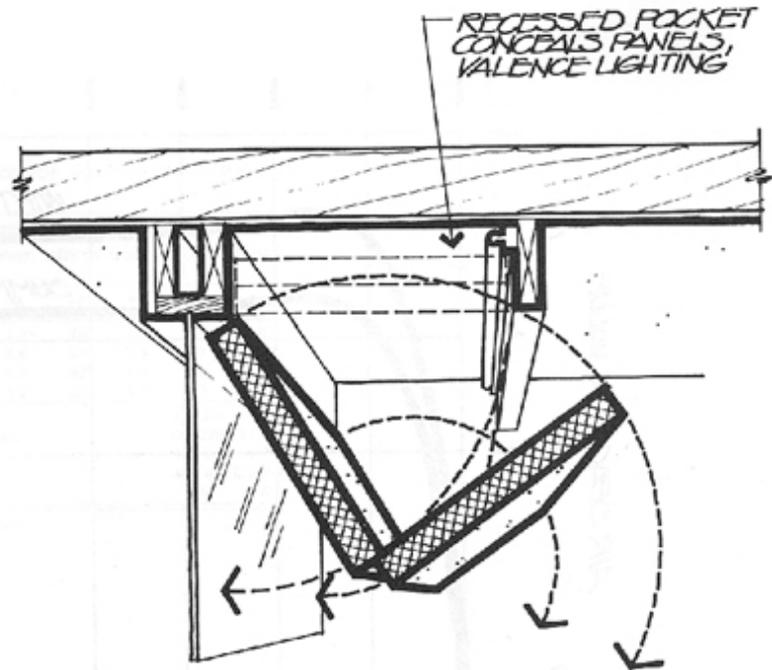
FIG. 39c. Hinged and fold-down panels offer large additional resistances to window units, can be made from aluminum-faced urethane or polystyrene sandwich panels, or insulation board w/laminated facings.
