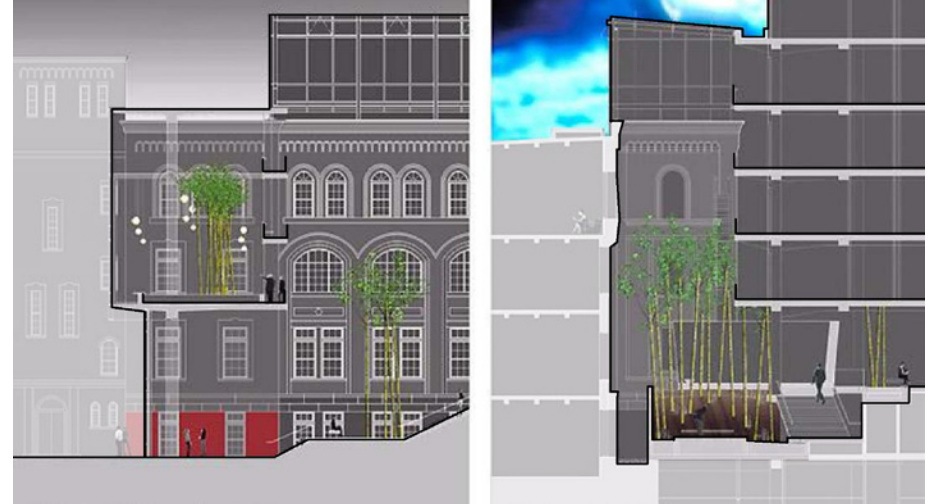
Figure 17 (Above Left): North-South Section of Winter Garden. Figure 18 (Above Right): East-west section of atrium. Figure 19 (Below): North-south section of atrium.
