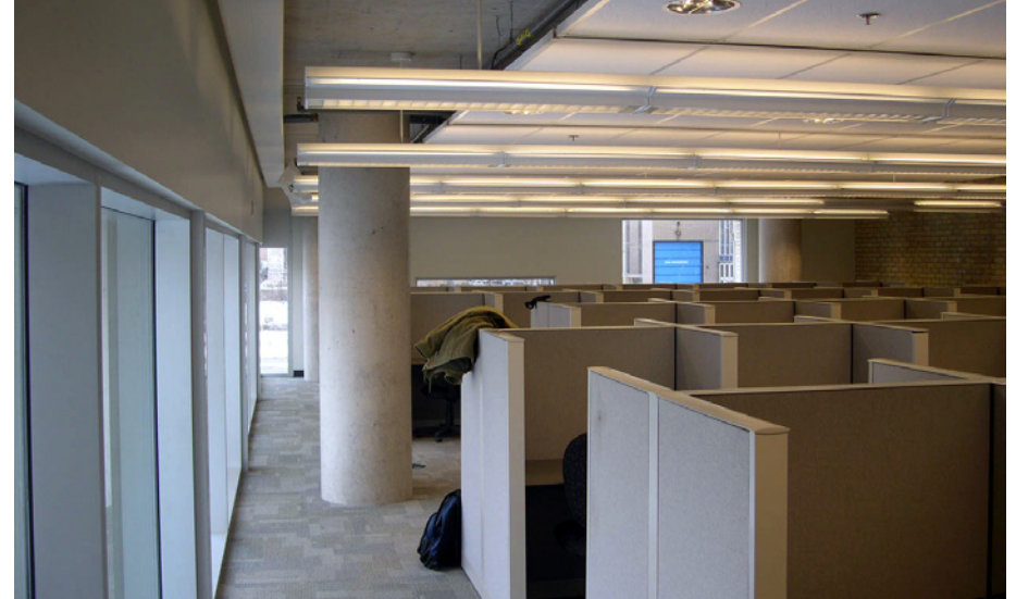
Figure 10 (Above): Interior partitions are low to allow light diffusion into spaces and moveable for increased flexibility. Figure 11 (Below): A glazed interior partition.
