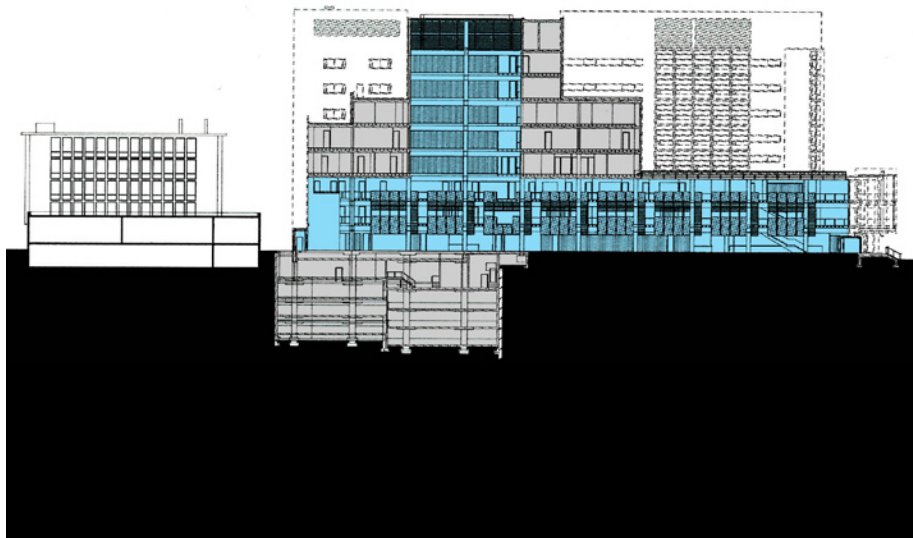
Figures 19 (Above): East-west section through the Bahen Centre atrium space. Figure 20 (Below): North-south section through the atrium corridor.
