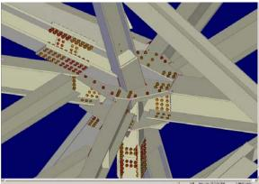
Figure: A single connection isolated in X-Steel
