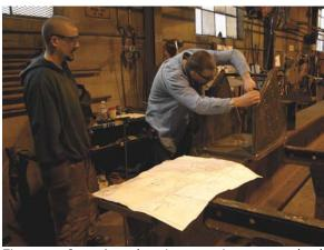
Figure 6: A drawing using standard orthographic projections sits aside the steel whose accuracy is checked with a carpenter's square, pencil and tape measure.
