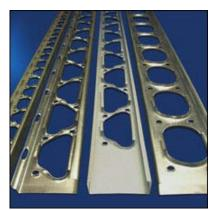
Fig 5: These steel studs, manufactured by Steelform Building Products, are available in widths to 200mm. Sprayed insulation can form around the metal, which has also been made thinner – possible due to the shaping of the material.
