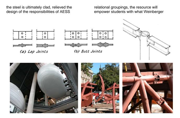
Figure 3. (clockwise from top left): Classic connection, detail from F. Ching of type of tube to W connection, detail of tube to tube connection with plate on the Leslie Dan School of Pharmacy, crane lifting pod segment for placement, and finished building – pods clad in gypsum board with painted finish
