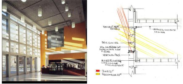
Displacement ventilation from below the raised floor and high level exhaust throughout the building provides up to 50% improvement in indoor air quality. Displacement ventilation air system is also installed below high occupancy rate auditoriums on the ground floor level.
