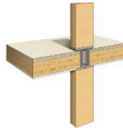
partial encapsulation during construction
